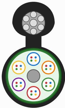
GYTC8S 3D Structural Illustration
